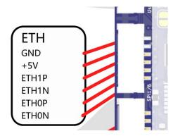
An important note must be made regarding the Ethernet connection. In order to allow Ethernet connectivity and without affecting the size of the ochin\_CM4v2 board, it was decided to adopt a transformerless configuration, like the one adopted and described by Texas Instruments in Application Note AN-1519 for their DP83848 Ethernet devices. It is therefore advisable to study and understand the AP-1519 before deciding to use the Ethernet port in a transformerless configuration.
